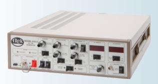
The Trek Model 615-3 is a precision high-voltage AC/DC generator that can be used in constant voltage, constant current or external amplifier mode. It is specifically designed to simultaneously provide the AC and DC operating potentials required to operate/control an electrostatic charger roller and offer features such as four-quadrant output, high rejection of load current noise and three wave output shapes.
